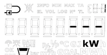
Error in the display of power as a result of a temperature sensor error
