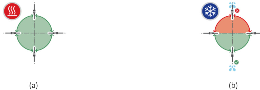
Figure 20. Acceptable orientation of a temperature sensor in (a) a heat and (b) a cooling installation.
