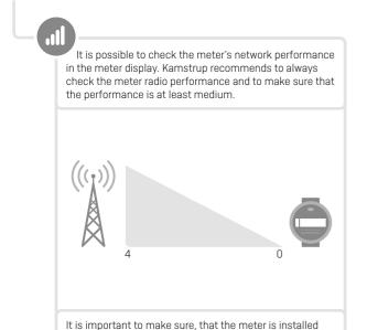
with the best possible radio performance to achieve maximum battery lifetime on the meter. If the meter is installed in poor radio conditions, e.g. in a meter well, it is recommended to check the network performance status.
