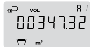
Figure 10: The meter's current count can be programmed into MULTICAL® as initial value by means of the PC-tool METERTOOL to allow accumulations to proceed synchronously.
