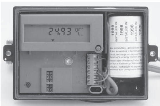
D-cell-litiumparistolla varustettu MULTICAL® Compact
