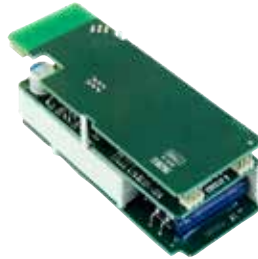
OMNICON® 4G module - 681Gxxxx with internal antenna.
