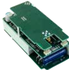
OMNICON® 4G module - 681Jxxxx with adapter PCB for external antenna.
