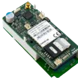
OMNICON® 4G module - 681Hxxxx for external antenna.
