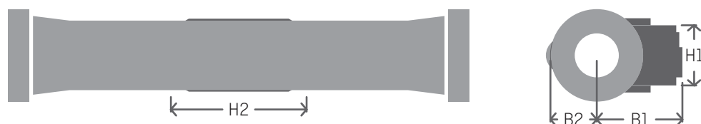
Figure 11: Flow sensor with G5/4 and G2 threaded connection
