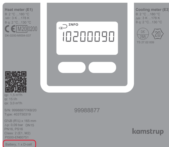
Figure 19: Correct position of label on MULTICAL® 403.
