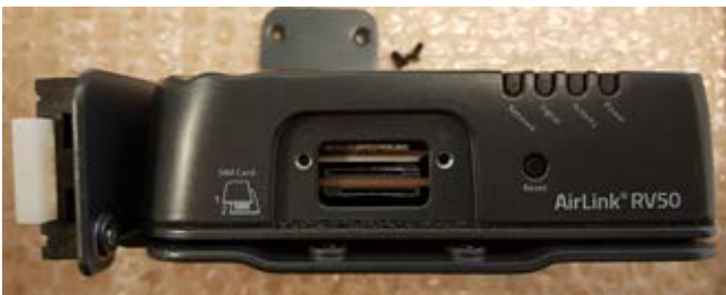
Figure 36 - SIERRA Wireless AirLINK RV50x, SIM installation 2
