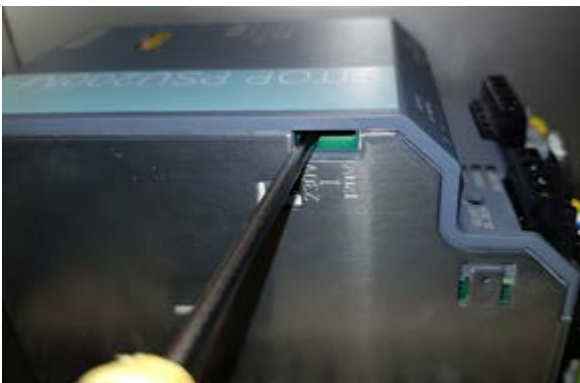
Figure 40 - READy Collector Base 230/120VAC switch
