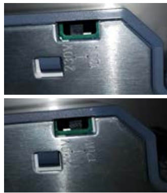
Figure 41 - READy Collector Base 230/120 VAC switch positions
