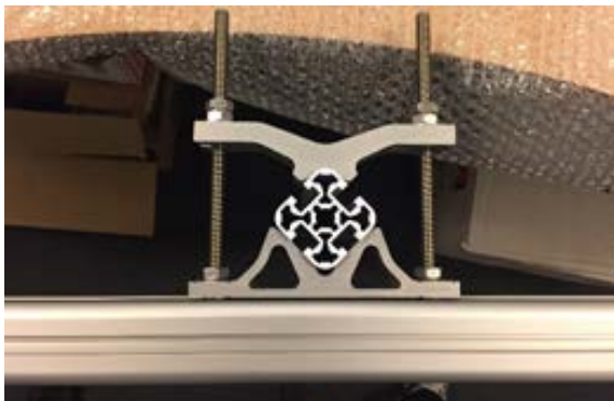
Figure 23 - Antenna beam bracket assembly installed
