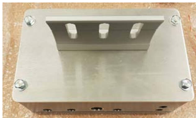
Figure 14 - Adaptor plate installed on READy Collector Top
