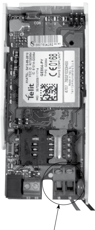
Load control output (max 230 VAC, 100 mA).
