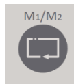
Figure 51. The left push-button shifts between readings/counts of the two flow sensor inputs. In the display, M1 and M2 respectively indicate the currently displayed flow sensor inputs/counters.
