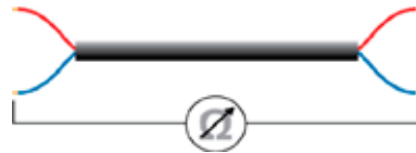
Measurement of cable resistance.
