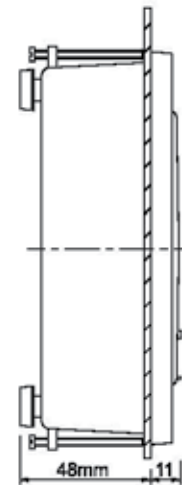
Panel mounted MULTICAL® Type 66-CDE, viewed from the side.
