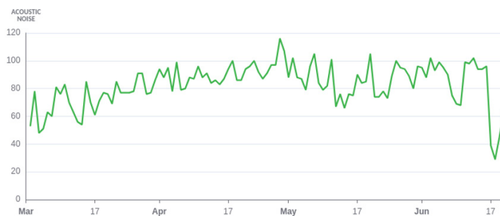
Example of a Leak Detector noise curve
