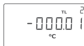
Figure 20: Setting up negative TL2 in "SETUP loop", the - will be flashing when on the sign position and stay on when moving to another decimal.
