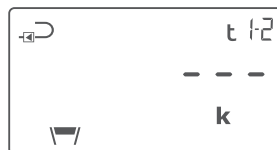
Reading of temperature difference t1-t2 at temperature sensor error
