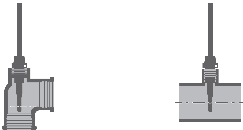
Figure 12: Examples of installation of sensor pocket for \varnothing 5.8 mm temperature sensor with R\frac{1}{2} thread (to the left) and sensor pocket for \varnothing 6.0 mm temperature sensor with G\frac{1}{2} thread and copper gasket (to the right).
