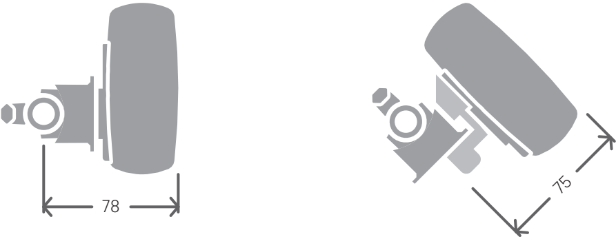
Figure 5: MULTICAL® 603 mounted on ULTRAFLOW® with G¼ threaded connection
