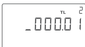
Figure 19: Setting up positive TL2 in "SETUP loop", the _ will be flashing when on the sign position but disappear when moving to another decimal.
