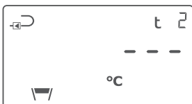
Reading of t2 in case of temperature sensor error
