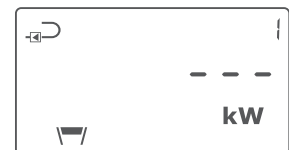
Error in power reading as a result of temperature sensor error
