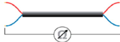
Measurement of cable resistance.
