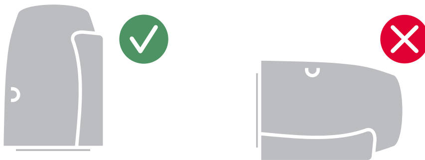
Figure 4 – READy 4G Bridge orientation
