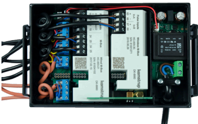
Wireless M-Bus module with internal antenna.
